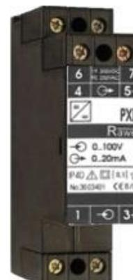
The module has been designed to convert DC current ( $\pm 50\mu\text{A} \dots \pm 10\text{A}$ ) or voltage ( $\pm 10\text{mV} \dots \pm 1000\text{V}$ ) from shunt resistors and sensors into a series of unified ranges (0..10V, 0..20mA, 4..20mA, 0..± 20mA, 0..±10V ). The converter output-to-input response is linear. The converter is particularly well-suited for heavy electromagnetic interference environment operation and features input-to-output isolation.
